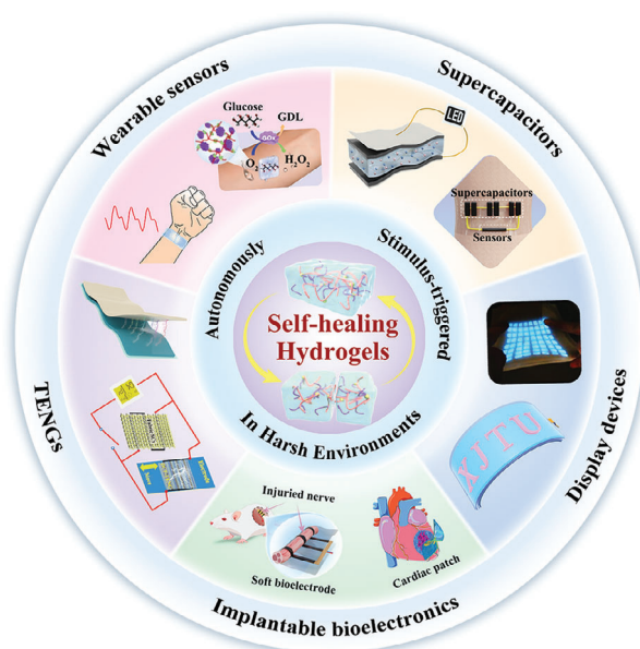
Figure 1. Schematic diagram of SHHs and their potential applications in soft bioelectronics. Wearable sensors: Reproduced with permission. [41] Copyright 2023, Elsevier. Supercapacitors: Reproduced with permission. [42] Copyright 2020, Elsevier. Display devices: Reproduced with permission. [43] Copyright 2016, American Association for the Advancement of Science. TENGs: Reproduced with permission. [44] Copyright 2020, American Chemical Society. Implantable bioelectronics: Reproduced with permission. [45] Copyright 2022, John Wiley & Sons. Reproduced with permission. [46] Copyright 2021, Elsevier.
